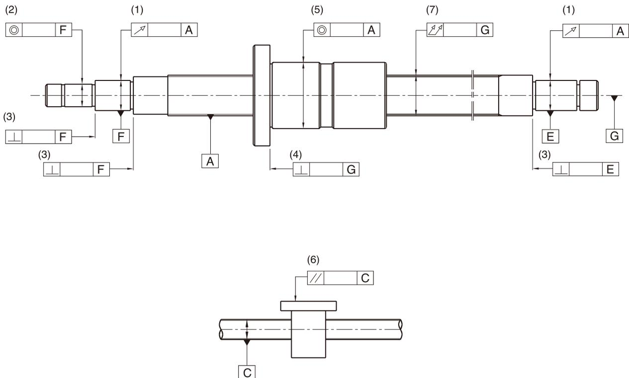
Fig. 2.2 Mounting Accuracy and Tolerances
