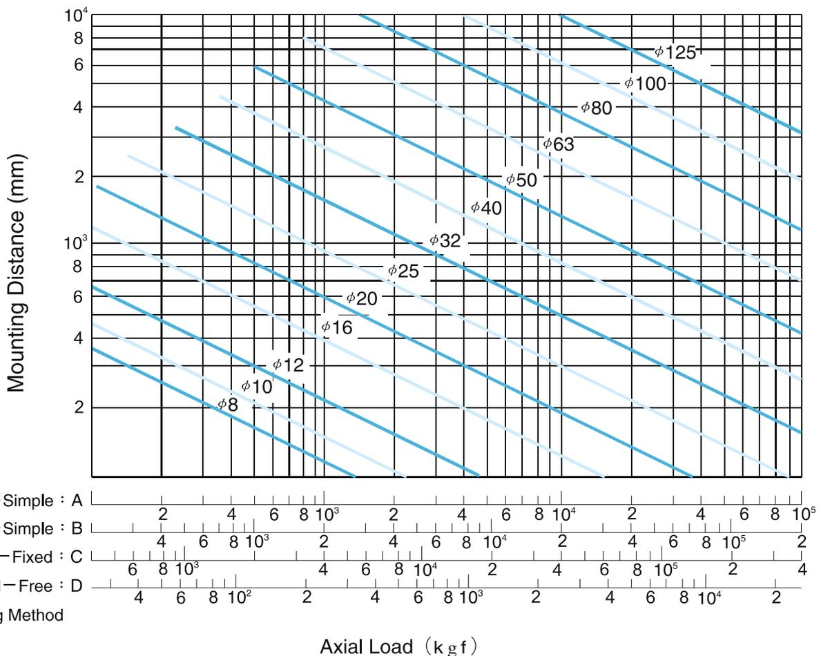
Fig. 3.16 Buckling Load vs. Shaft Dia. and Length
