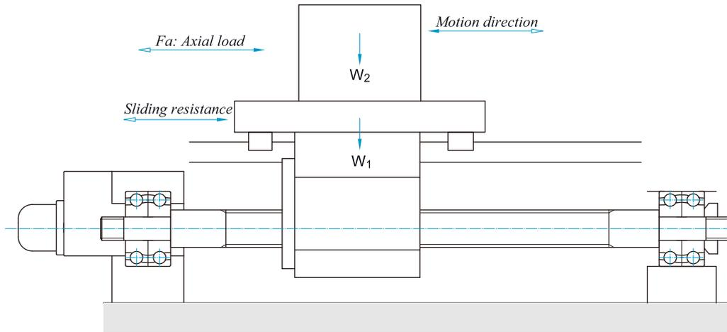
Fig.4.9 Horizontal reciprocating moving mechanism
