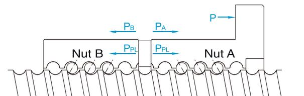
Fig. 4.6 Preloaded for the double nuts
