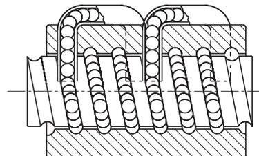
Fig. 4.2 External ball circulation's nut
